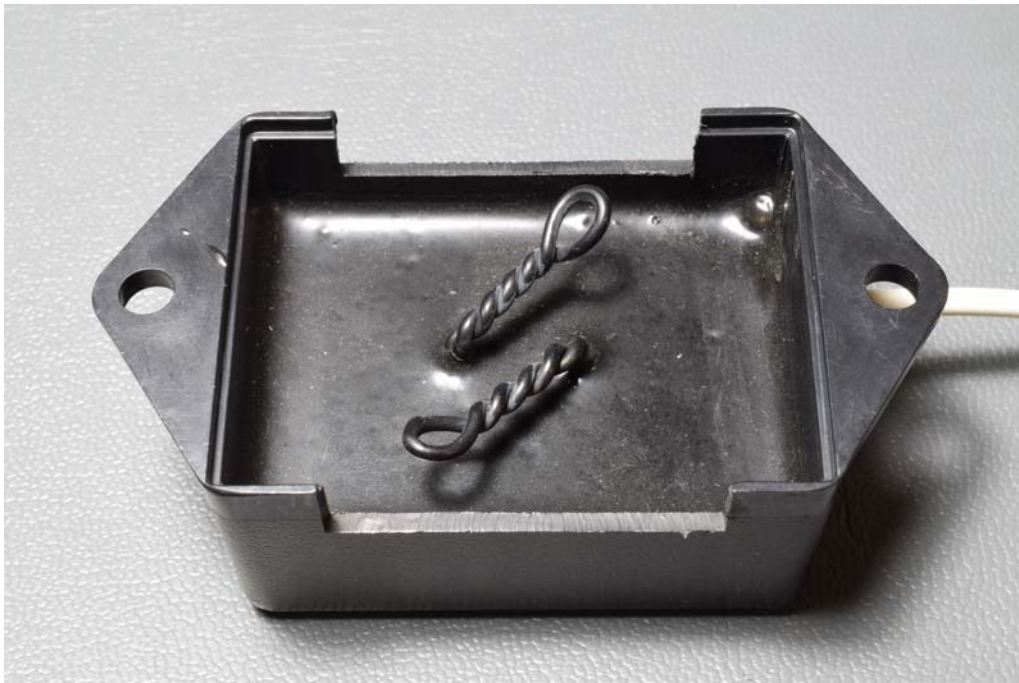
Figure 4: Close-up photo of the C5001 water sensing spot detector showing its twisted pair of detection wires. Water is detected when it covers the two twisted pair wires.
