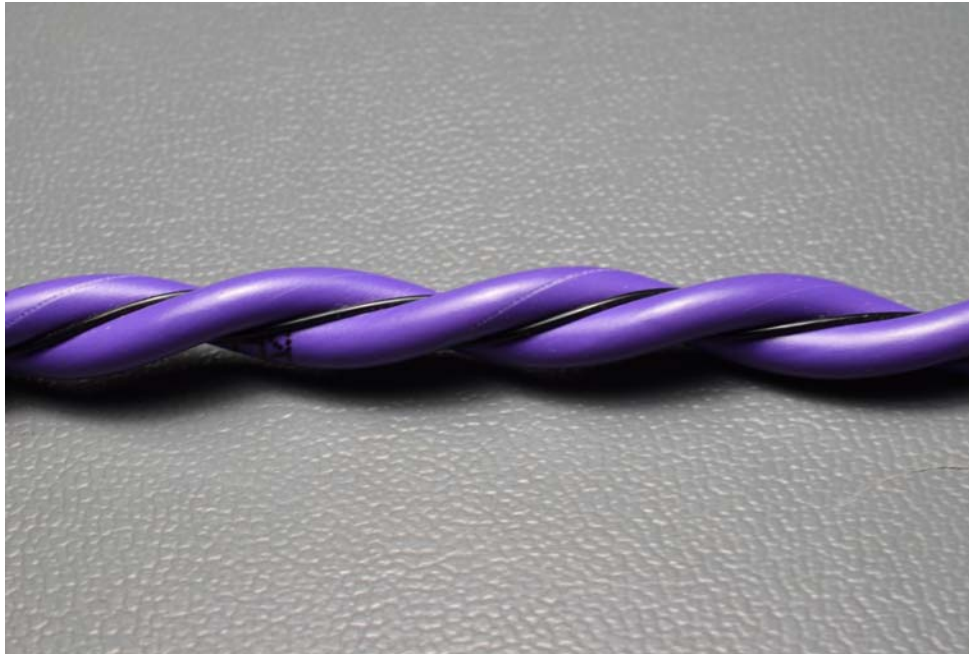
Figure 3: Close-up photo of the C5000 water sensing cable showing its purple colored substrate and black pair of interleaved water sensing wires. Water is detected when it covers the pair of black wires.
