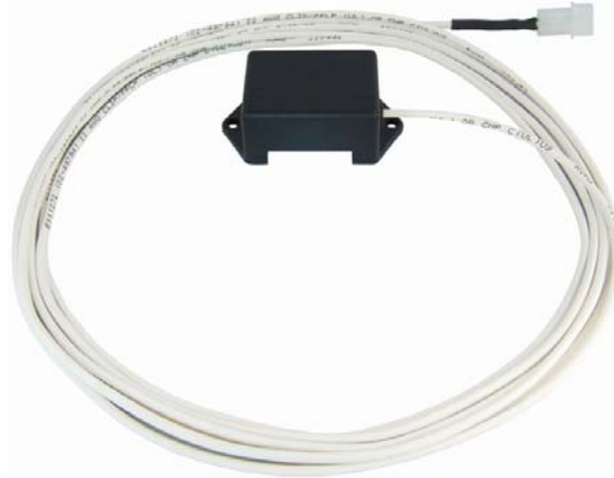
Figure 2: Photo of the C5001 water sensing spot detector. It has a two pin electrical connector and white (14 foot) lead-out cable that plugs into the SS6201J communications module. Two mounting holes allow the C5001 to be fastened down with screws or rivets.
