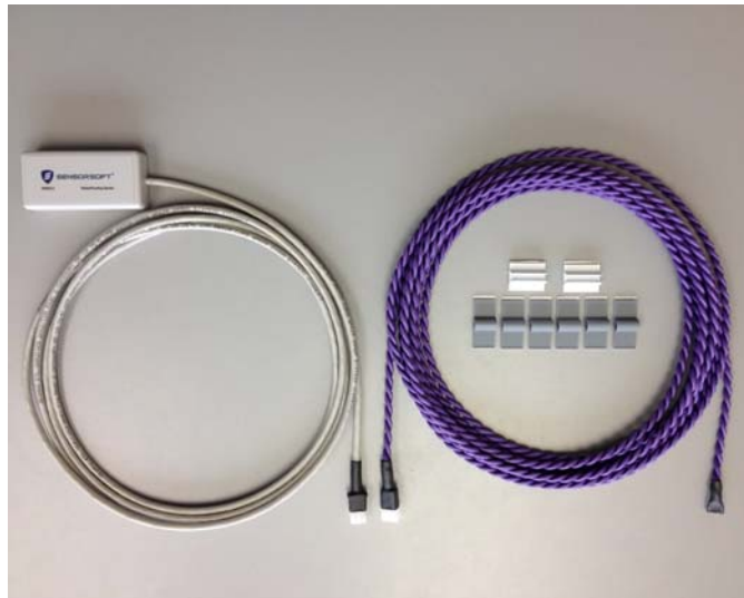
Figure 1: The SS6201J communications module with 10 foot gray lead-in cable (left) and C5000 20 foot purple water sensitive rope cable (right). A two position connector is used to connect these products together after installation. Included plastic adhesive fasteners (F1005) are provided to install the C5000 rope cable to most surfaces.
